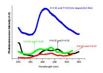
**Fig: 3.** Photoluminescence emission spectra of undoped ZnO film and Co(x = 0.04, 0.03, 0.02) and Al(y = 0.01, 0.02, 0.03) doped ZnO nanostructured films for better comparison of intensity of photoluminescence.
