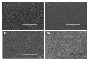
Fig: 2(a-d) SEM surface morphology of undoped ZnO and Co(x =0.00, 0.04, 0.03, 0.02) and Al(y = 0.00,0.01, 0.02, 0.03) doped ZnO nanostructured films, (a) undoped ZnO film, (b) Co(x = 0.02) and Al(y = 0.03) doped ZnO film, (c) Co(x = 0.03) and Al(y = 0.02) doped ZnO film, (d) Co(x = 0.04) and Al(y = 0.01) doped ZnO film
